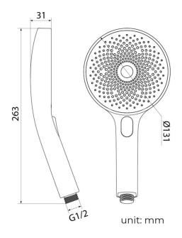
Flow Rate: 2.0 GPM / 7.6 LPM
